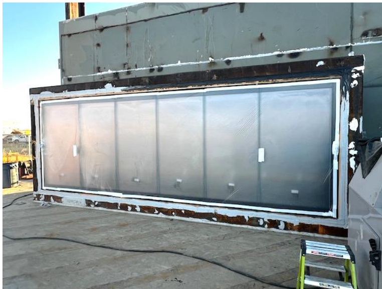
Photo No. 2 Test Specimen during Air Infiltration
