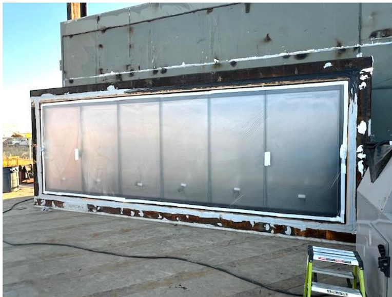
Photo No. 2 Test Specimen during Air Infiltration
