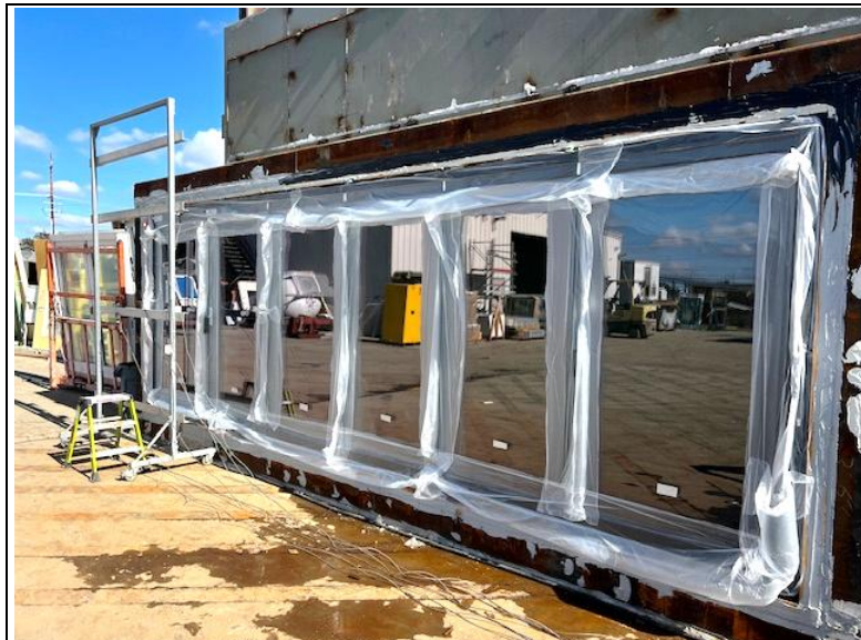
Photo No. 3 Test Specimen during Structural Wind Loading
